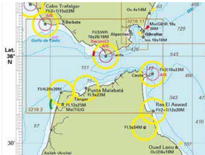
Real (or Physical) AIS located at physical AtoN
