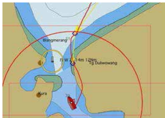
Satellite yacht track graphics to illustrate chart offsets
